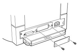
2. Align the edges of the 3000E board with the rails in the interface slot and slide the 3000E into the printer. Secure with the two screws removed in Step 1.
